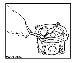
1. Clean the filter cover to prevent dirt from entering tank.
